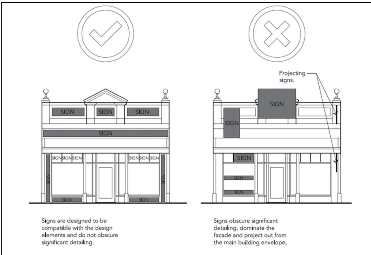
Figure 9 - Examples of appropriate and inappropriate signage. Griffiths Architects 2015
